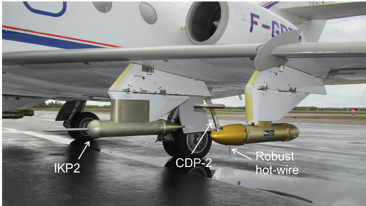
Figure 5. Photograph of two core instruments of the campaigns mounted under the wing of the Falcon-20: the isokinetic evaporator (IKP2) reference TWC instrument, and the DMT CDP-2. The SEA Robust hot-wire TWC probe is also shown. The core SPEC-2D-S and DMT PIP probes are partially visible in the background under the other wing. See also Figs. 6-7.
