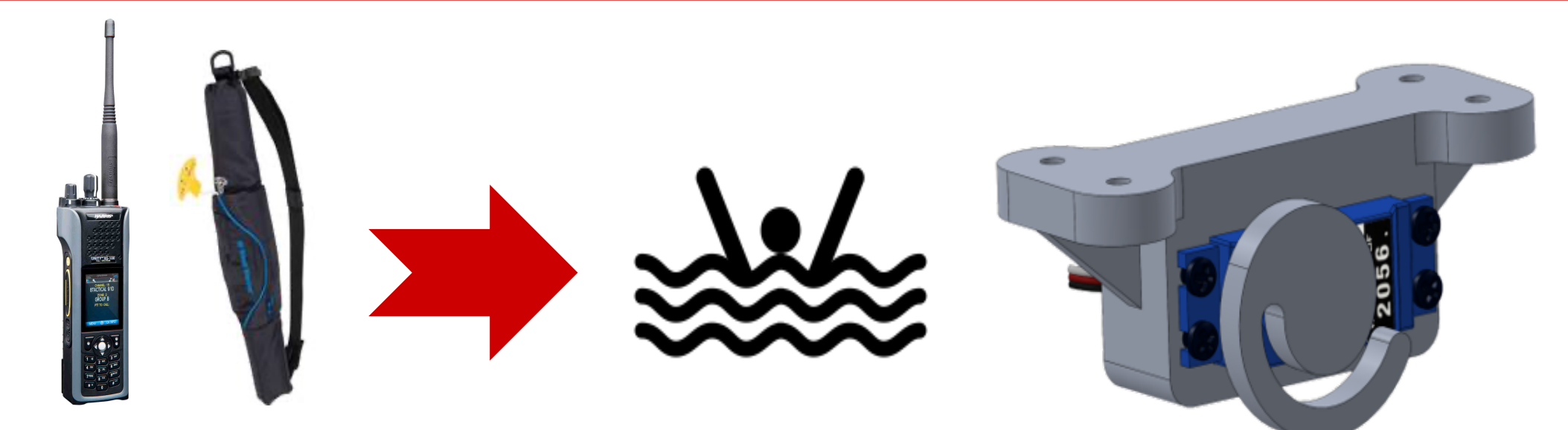
Figure 4: Payload components. (Left) Two-way radio and Type-5 PFD are deployed in rescue operations via (Right) servo-actuated spiral hook mechanism
