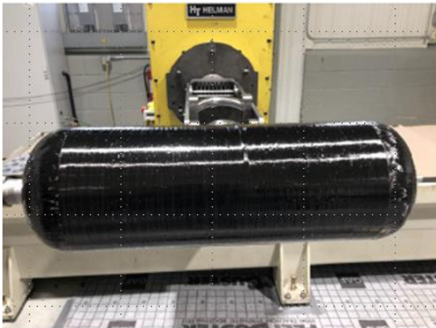
Figure 7.2.3-3. Wrapping of the liners with the composite [ref. 15].
