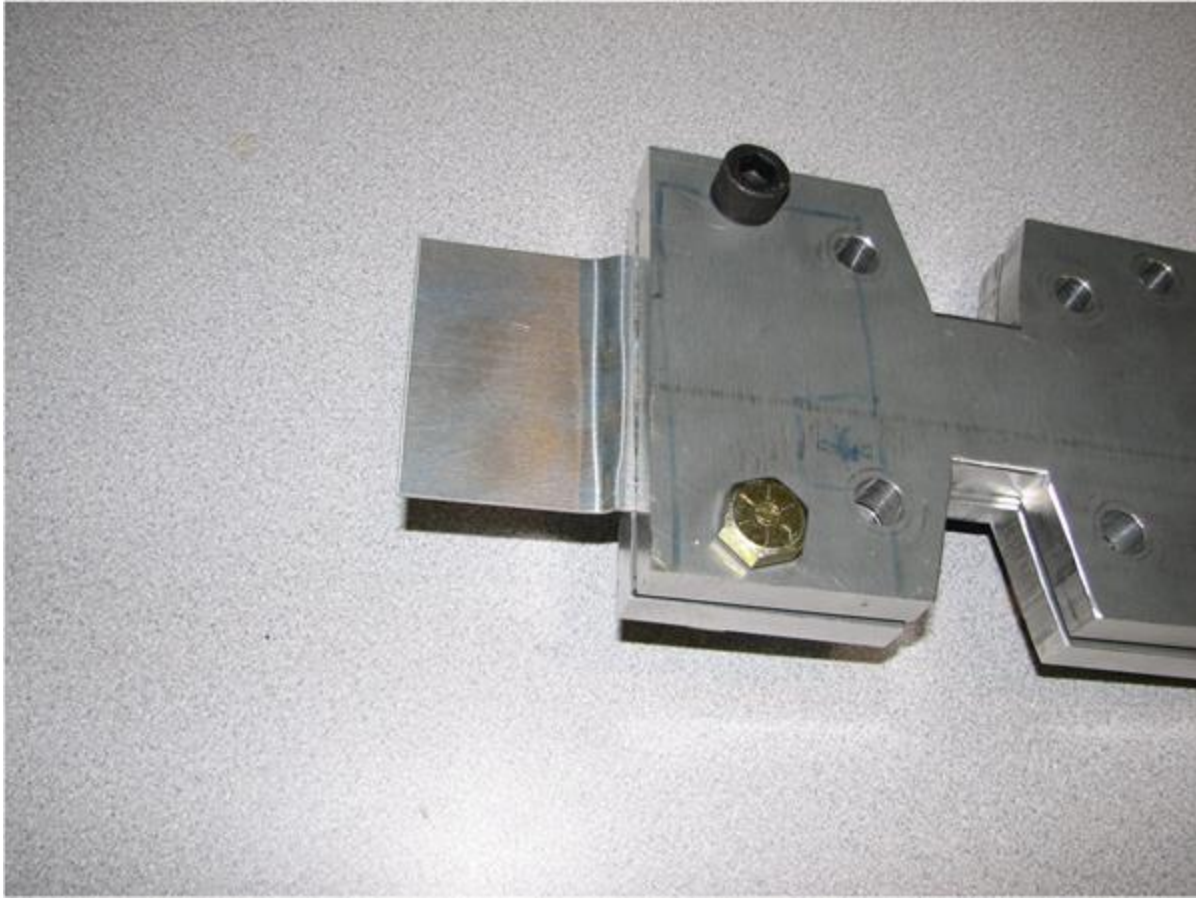
Figure I.2. Example of coupon buckling at the gap between the guide plates and the grips [ref. 1].
