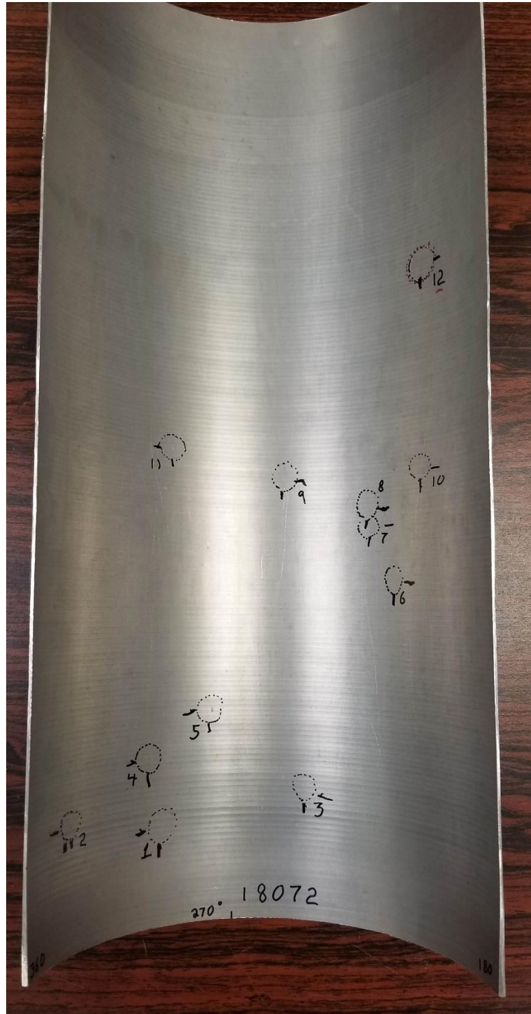
Figure K.17. Marked section of liner 18072 following high frequency ID Eddy Current inspection.
