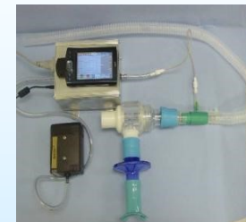
Hydrazine EVA Sensors (ppb Level Detection)
