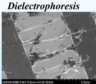
TiO 2 Nanorods aligned by dielectrophoresis across interdigitated electrode patterns.
