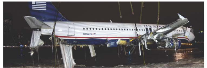
(b) Photograph of A320 aircraft damage.
