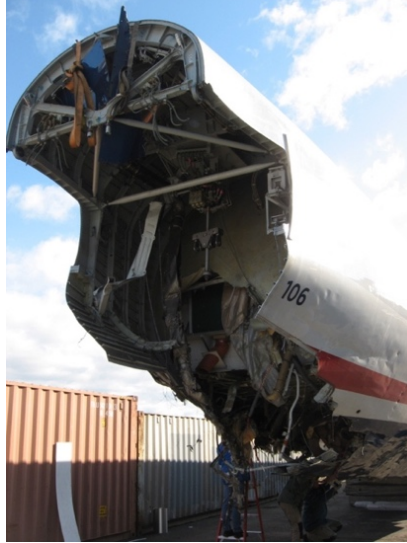
(c) Tail section of the A320 after removal of damaged parts.
