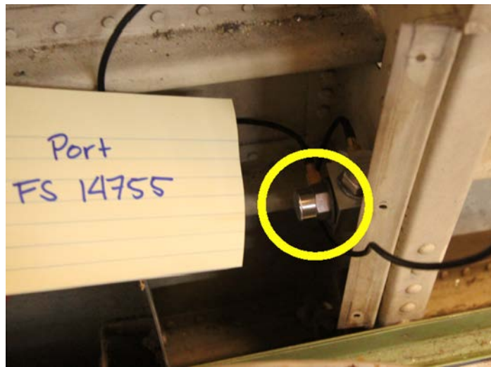
Figure 16. Photo of an airframe accelerometer, that was used in the 2019 crash test of the F28.
