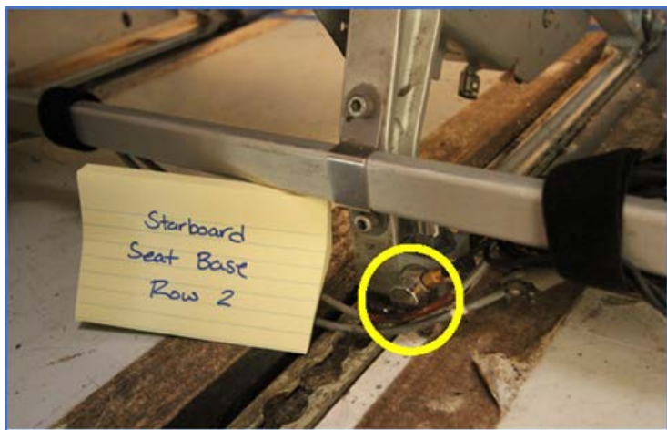
(b) Photo of a typical seat base accelerometer used in the 2019 crash test of the F28 onto soil.
