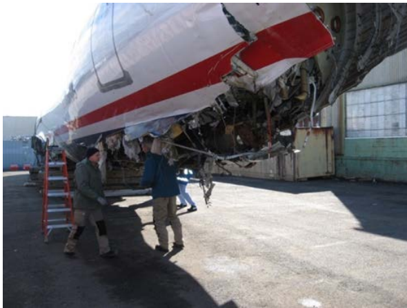
Damage to the tail section, looking forward.
