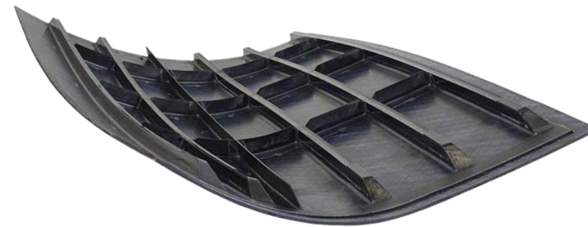
Double curvature. The thermoplastic composite fuselage panel accommodates the complex geometry of a Gulfstream business jet aft fuselage with fiber-steered AFP layup of the skin and co-consolidation of the orthogrid. Note the circumferential blade stringers, which are later welded to the frame. Image Courtesy of Fokker GKN.
