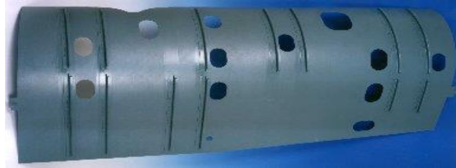
Dassault Rafale Engine Tunnel Stiffeners Welded to Skin APC-2/AS4
