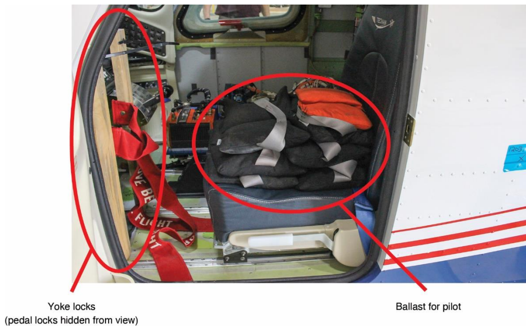
Figure 7: Yoke locks and pilot ballast setup inside the cockpit for the X-57 Mod II ground vibration test
