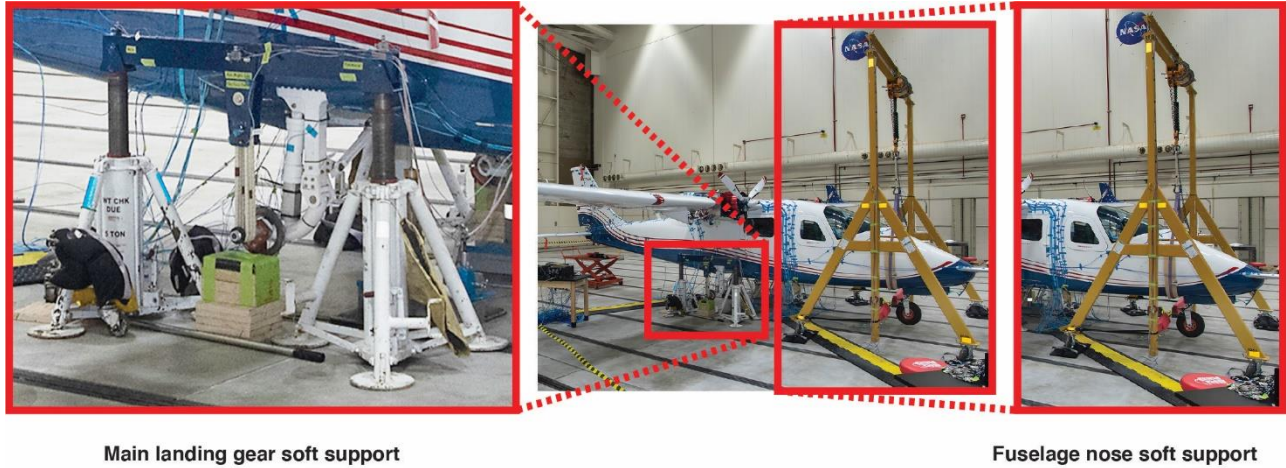
Figure 10: The soft-support system used for the free-free boundary condition setup
