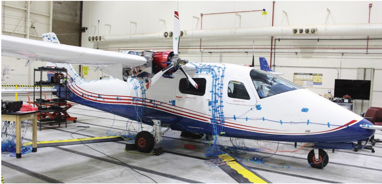
Figure 11: On-tires boundary condition setup
