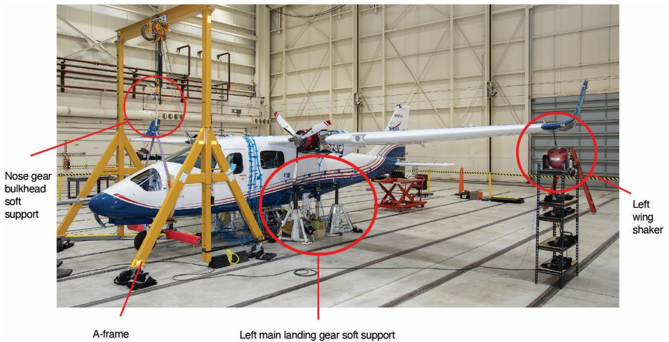
Figure 3: X-57 Mod II airplane ground vibration test setup on soft supports to simulate a free-free boundary condition
