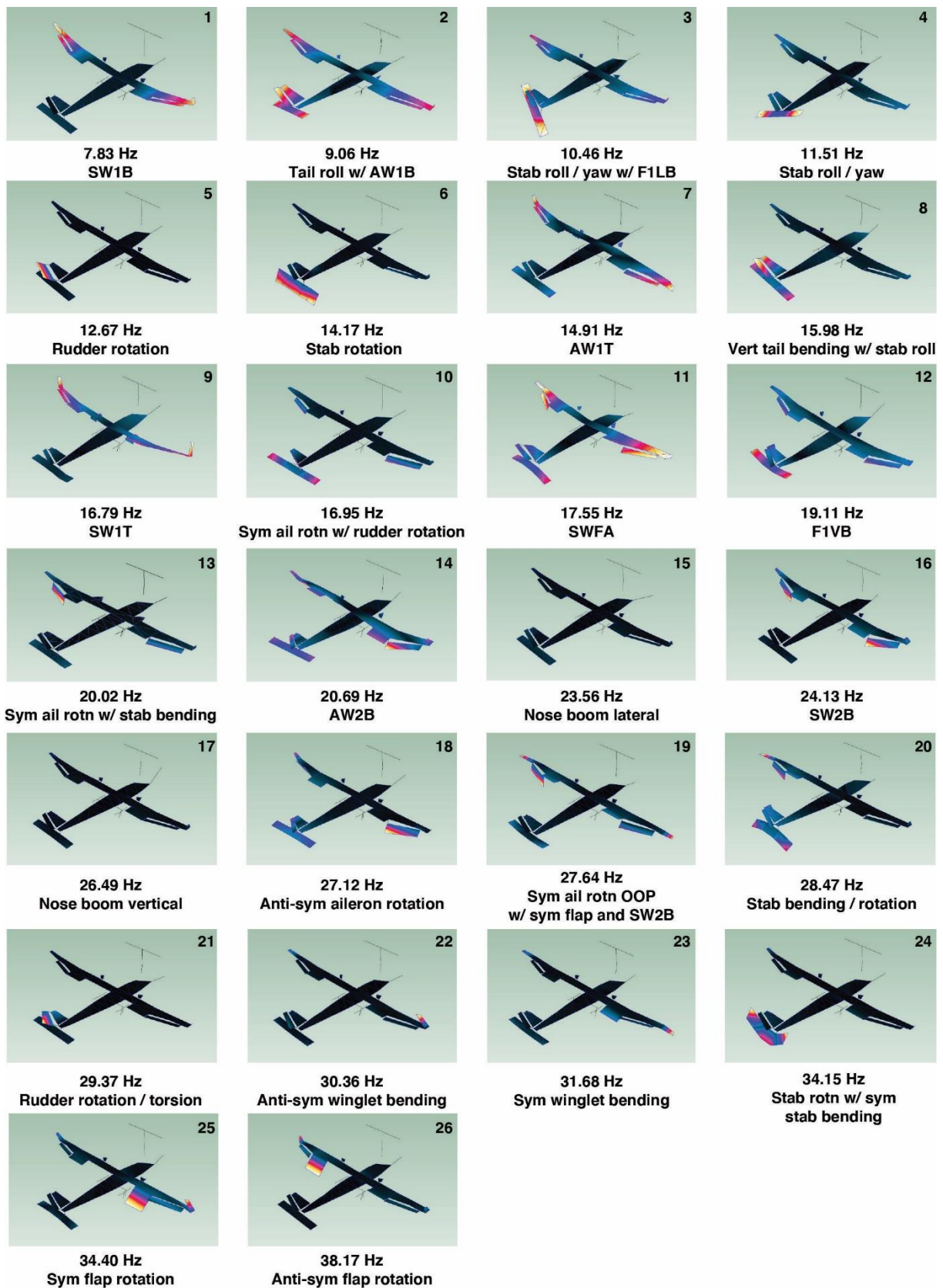
Figure 19: Ground vibration test airplane mode shapes for the free-free stab counterweight off setup shown in the order presented from Table 3
