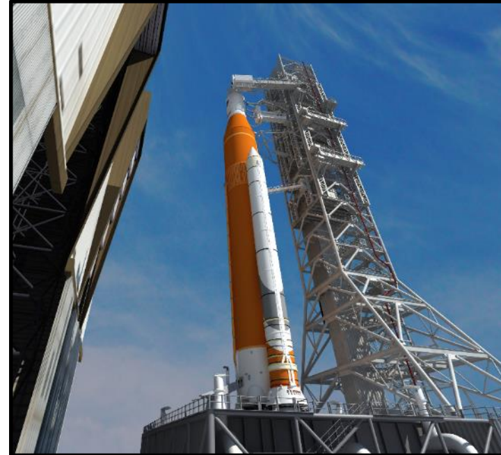
Artist Concept of Orion, Space Launch System (SLS), and Mobile Launcher (ML) Rolling Out of VAB
