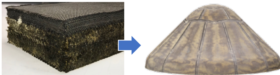
Figure 1. HEEET dual layer dry weave (left) and 1-meter Engineering Test Unit (right).
