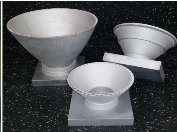
40" dia and 38" height nozzle with internal features built in 30 days using BP-DED
