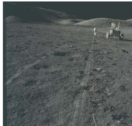
Fig. 3. Apollo 17 astronaut Jack Schmitt deploys an antenna for the Surface Electrical Properties (SEP) experiment. Analogous operations are required for MT. AS17-134-20436.
