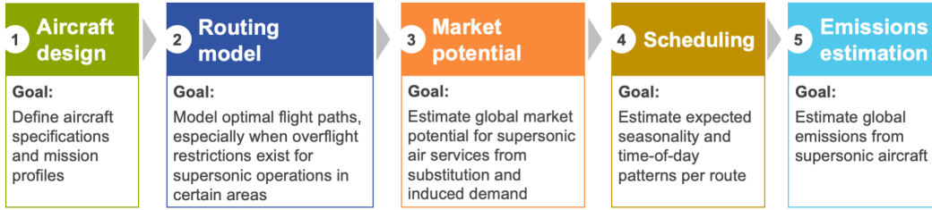
Figure 1: Modeling steps for deriving market and emissions scenarios for supersonic aircraft.
