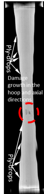
X-Ray CT images showing location, size and mode of damage
