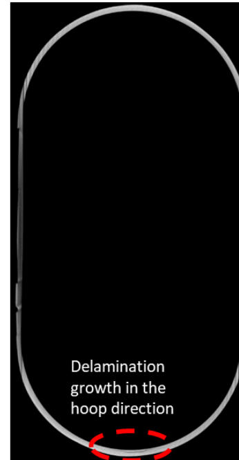
X-Ray CT images showing location, size and mode of damage
