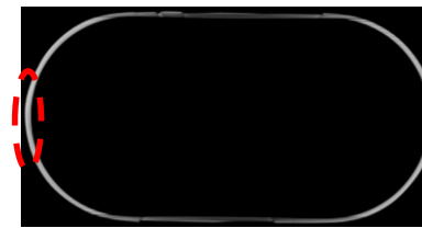
Observed and Predicted Damage Morphology after 40,000 Torque Cycles
