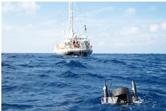
Fig. 2. Measuring reflectance by measuring below water upwelling radiance and downwelling irradiance and propagating the measurement above the surface.
