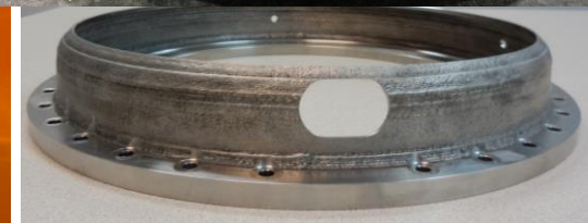
Bimetalllic Nozzle with L-PBF and DED (RAMPT Project)
