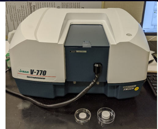
The reflectance spectrometer and two solar white samples.
