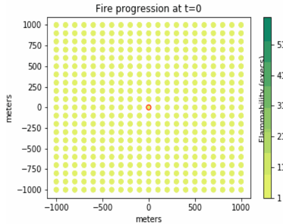
Figure 3: Fire propagation on a uniform map with no wind. Animation provided in level_fire_verification.gif.
