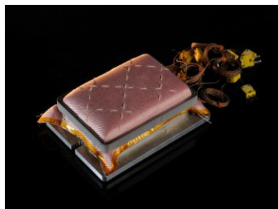
Test specimen with thermocouples
