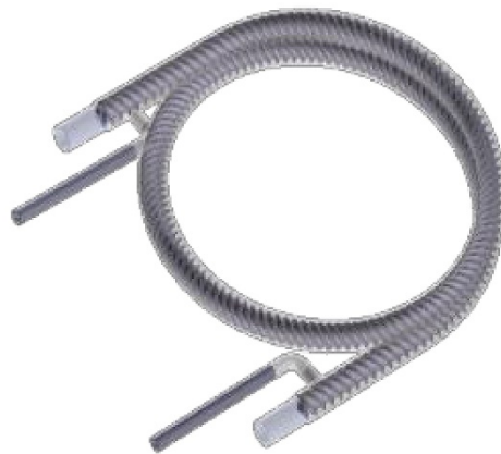
Figure 4.—Conceptual drawing of the Condenser, spiral finned inner tube visualized through the outer tube.
