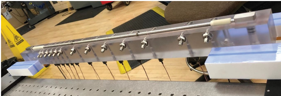
Figure 19.—Braided tube installed in the lower polycarbonate piece of the Condensation Test Module 1.
