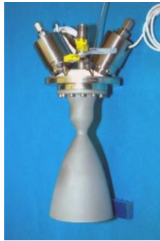
Figure 3. 100-lbf LOX/CH4 Thruster
