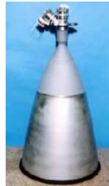
Figure 7. R-4D-11 with 300:1 Expansion Ratio
