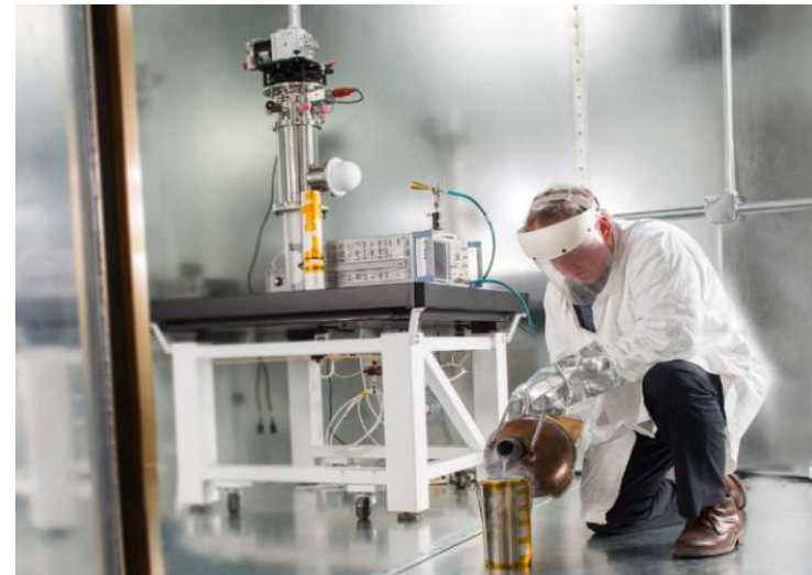
Inside the Superconducting and Cryogenic Microwave Electronics Laboratory at NASA Glenn. The room is shielded from electric and magnetic fields for conducting extremely sensitive receiver measurements. The customized 4K closed-cycle refrigerator is equipped with a microwave transparent Beryllia radome in this photograph
