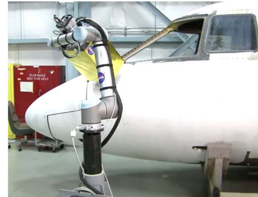
Robotic inspection on a fuselage
