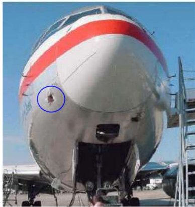
Bird strike impact damage
