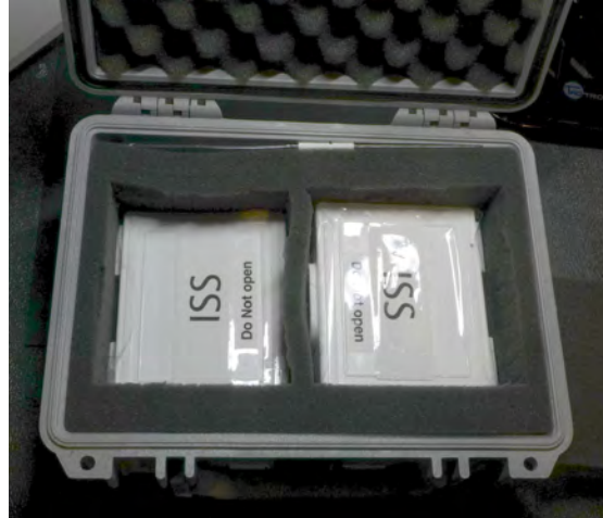
Figure 3. Opened ISS case showing two cassettes holding HELIOS test media.
