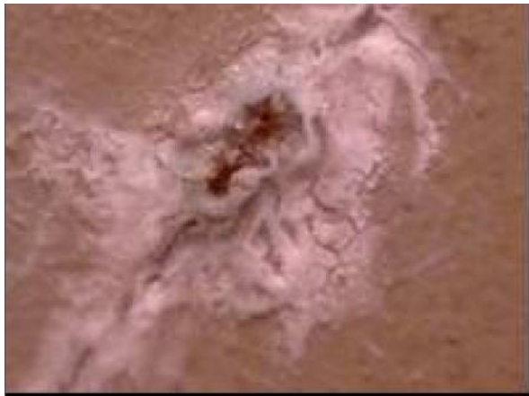
Enterprise Panel Scribe Pitting @ 60X mag After 500 hours
