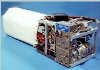
Space Shuttle Fuel Cell (1979 - 2012)
