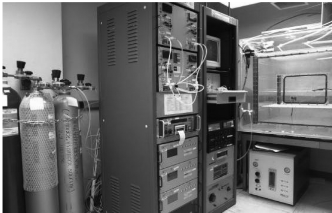
Figure 10.3 MFG chamber located at CALCE at the University of Maryland.
