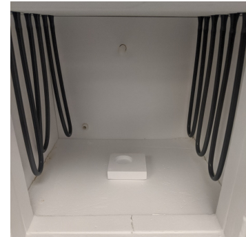
The inside of the new oven, allowing higher sintering temperatures. A ceramic mold containing pressed powder is shown.
