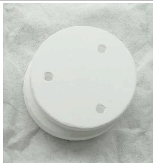
Rigid tile coating with holes for suspension in test chamber
