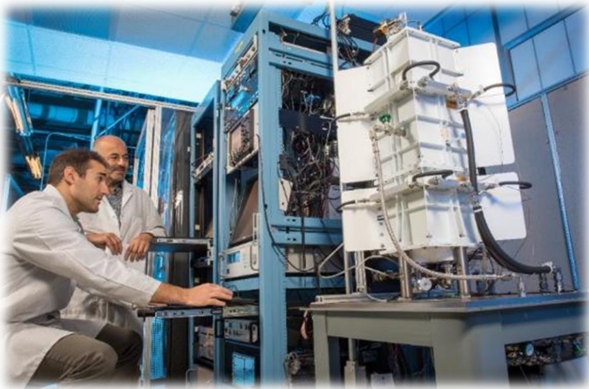
Electrically-heated DRPS test station at NASA GRC
