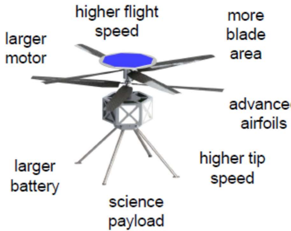
Figure 33. Improvements of a small MHH vehicle as compared to the Ingenuity Mars Helicopter Technology Demonstrator
