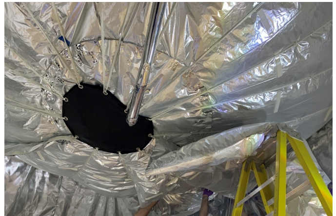
Figure J.14.—Installation of second subblanket on aft dome.
