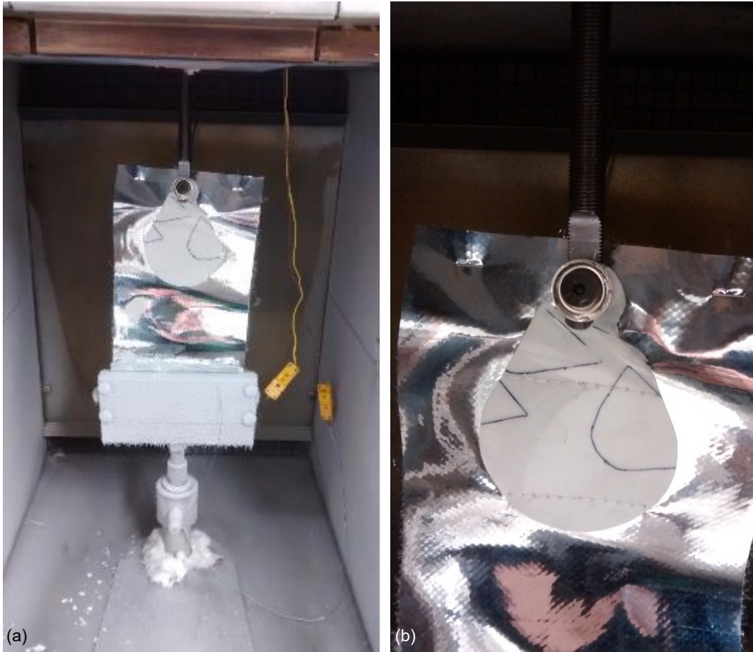
Figure J.5.—Structural coupon after testing. (a) Coupon in fixture. (b) Damage after testing.
