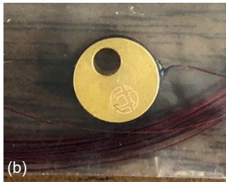
Figure 17.—Silicon diode (Scientific Instruments, Inc., Model 410AA). (a) Canister style. (b) Bobbin style.
