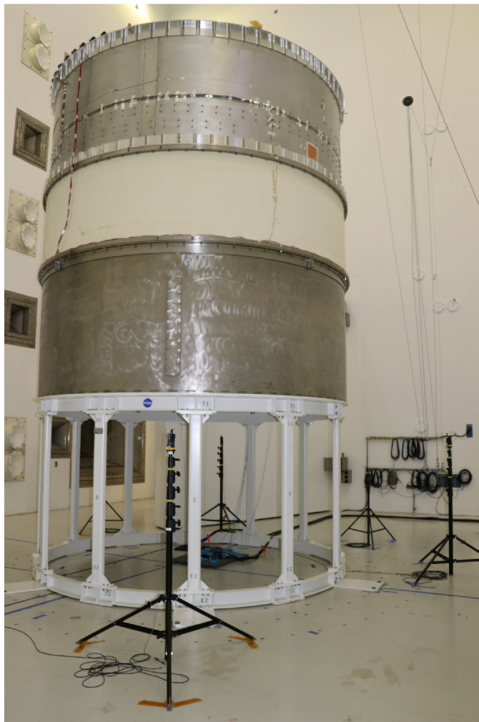
Figure 118.—Structural Heat Intercept, Insulation, and Vibration Evaluation Rig (SHIIVER) in Reverberant Acoustic Test Facility (RATF). Microphones are located on tripods.
