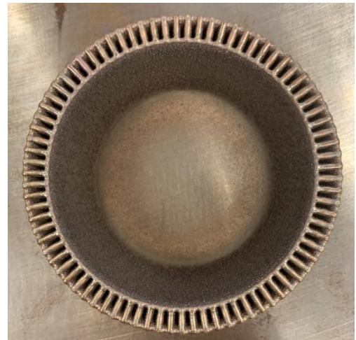
FIGURE 1: CROSS SECTIONAL VIEW OF A CHANNEL-COOLED MCC
