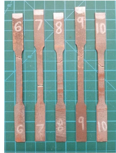
FIGURE 10: TENSILE SAMPLES AFTER TESTING
