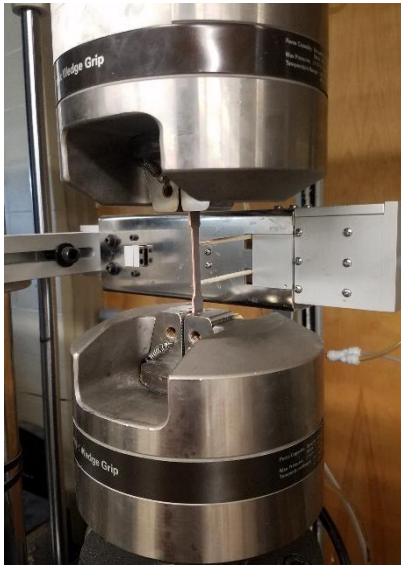
FIGURE 8: TENSILE TESTING SETUP
