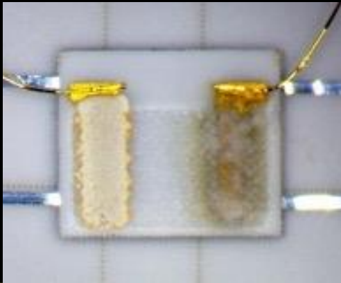
Makel Chemical Sensor Testing in GEER
