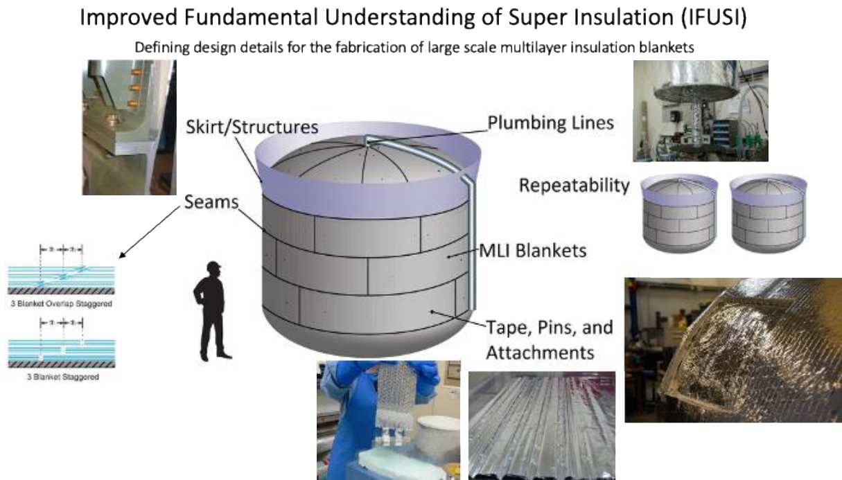
Fig 1. IFUSI performed thermal characterization testing on MLI systems, epoxies for cryogenic tanks, and assessed thermal repeatability of MLI systems.
