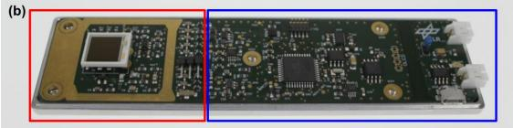
**M-42 upcoming mission:** Within the NASA Artemis I mission 16 M-42 detectors will be mounted within the two female phantoms HELGA and ZOHAR to record the radiation dose these phantoms receive on the way to and back from the Moon.
