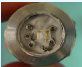
Sensor element mounted in custom A/N fitting
