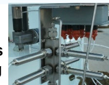
Sensor probes in emissions testing rig manifold
