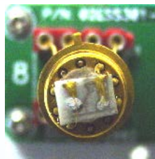
Lithium phosphate based CO 2 sensor
