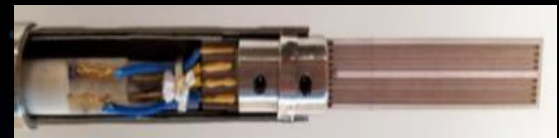
Drag force anemometer (wind sensor)
