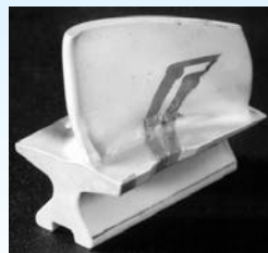
PdCr strain sensor to T=1000°C
