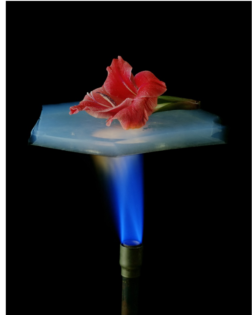
Bunsen burner applied to aerogel (LANL)
