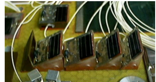
Tilted solar cells, to test rate of dust accumulation as function of tilt angle.
