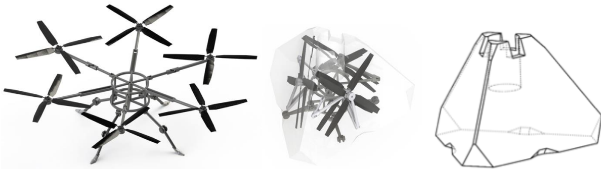
Fig. 6. Hexacopter for the Pathfinder lander, folding arms (Layered A design).
