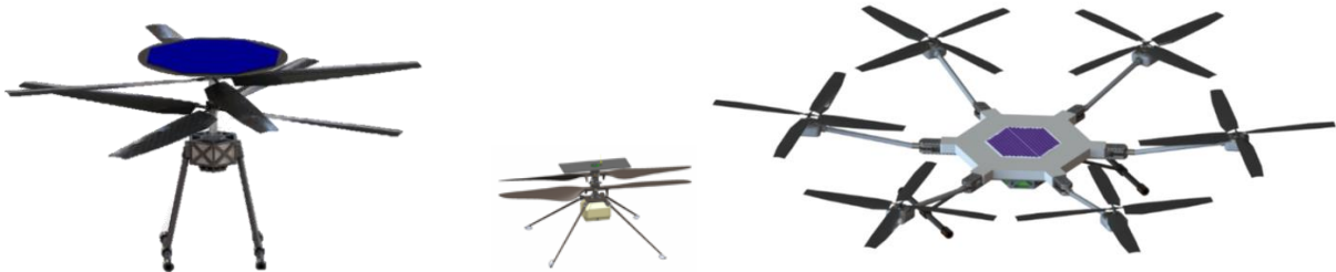
Fig. 4. Mars Science Helicopter configurations, with Mars Helicopter (center) for scale.
