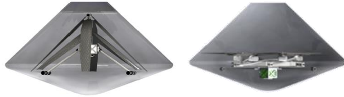
Fig. 5. Droop fold (co-axial) on left and rotating arm fold (hex) on right.
