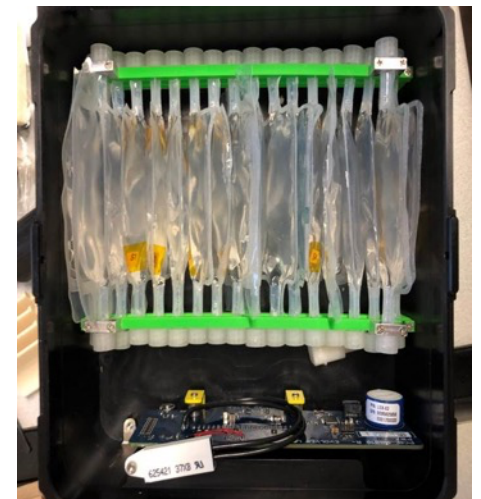
Pumps, bags & valves in multiple sizes with 24-bag configuration shown on right.
