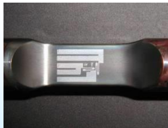
PdCr thin film strain gauge applied to a material sample for disk life fatigue testing
