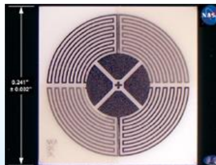
Heat Flux Sensor Array to T=1000^{\circ}\text{C}
