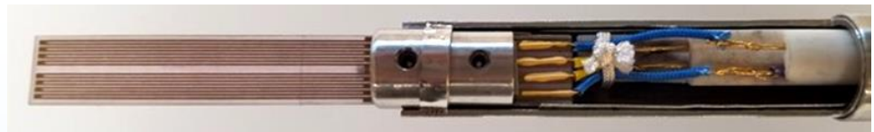
LLISSE Wind Sensor Proof-of-Concept (above)
