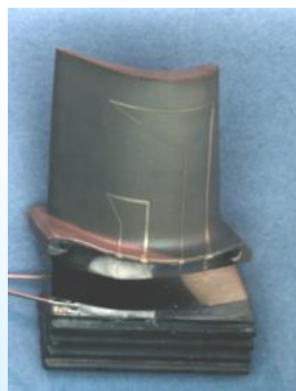
Pt- Pt/Rh temperature sensor to T=1200^{\circ}\text{C}
