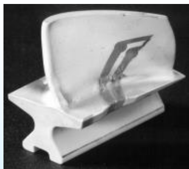
PdCr strain sensor to T=1000^{\circ}\text{C}
