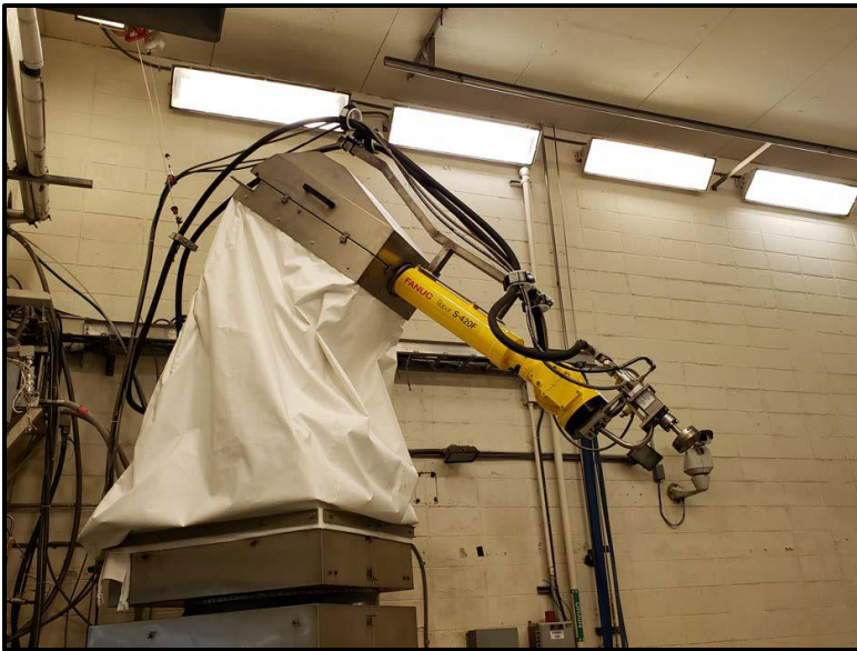
6 Degree-of-Freedom Robot Used for Automated Cleaning
