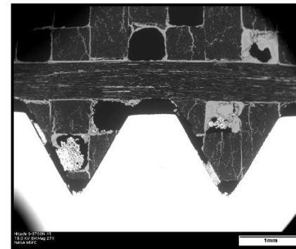
C/C-SiC threaded component examined under scanning electron microscopy (SEM) as part of postflight test hardware assessment for Orion LAS.
