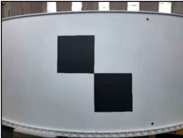
MSA with EM41-Developed Black Target and White (accreage) ESD Coatings Applied
