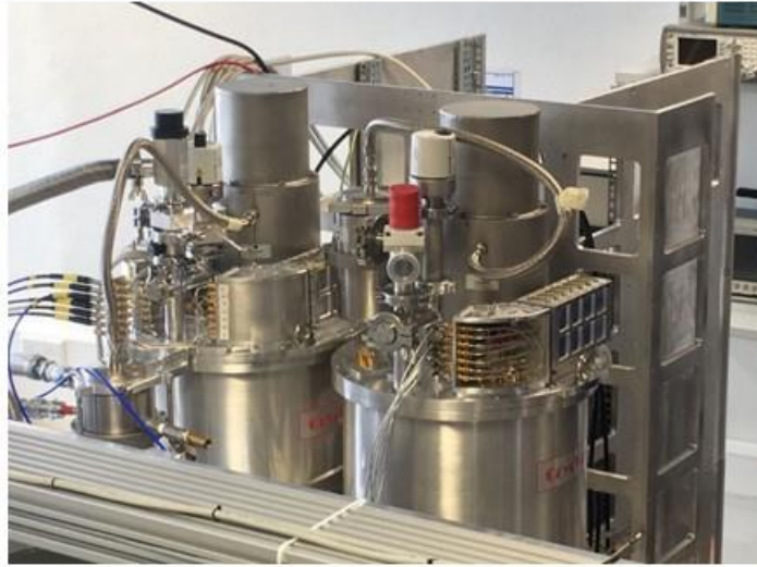
Figure 5.6-2. Left: GREAT SI prior to mating with the Telescope Assembly (TA). Right: Two PT-cooled cryostats installed. (Heyminck, 2018).
