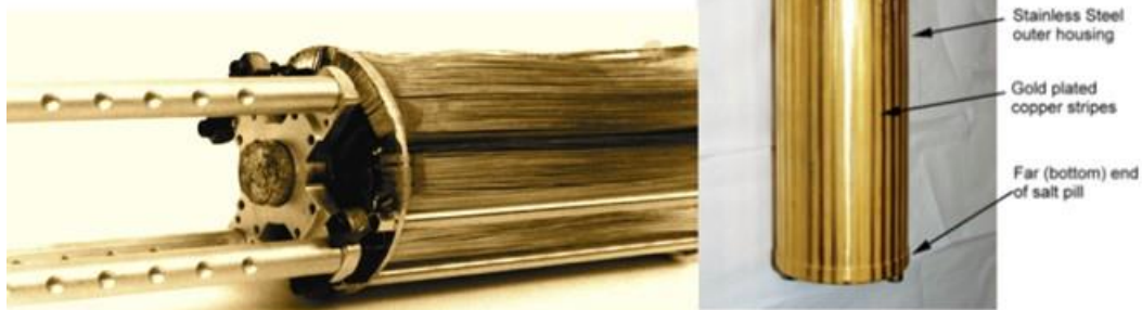
Figure 8.16-1. ADR salt pill manufacture.
