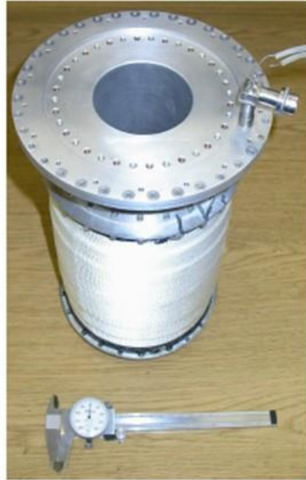
Figure 8.18-1. XRS ADR. Left: the salt pill removed from the bore of the magnet; Right: Superconducting magnet made by Cryomagnetics, Inc.
