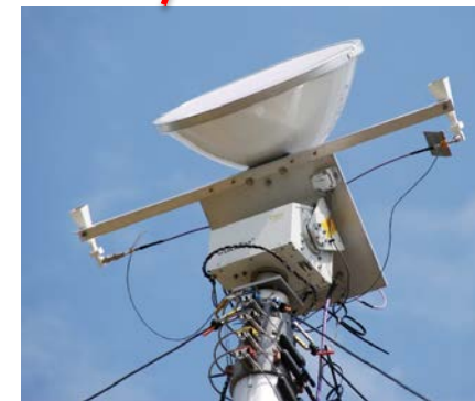
Ku-Band Multi-Polarization Receive Antennas
