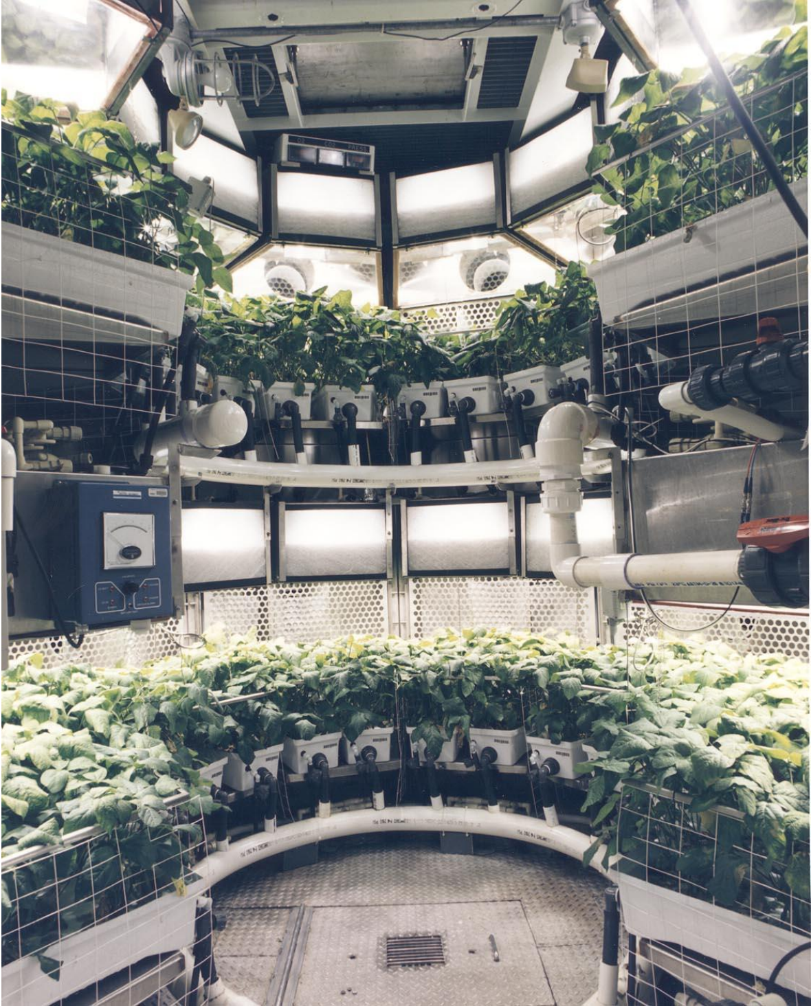
Figure 2. NASA's Biomass Production Chamber at Kennedy Space Center with a soybean crop. Two of the four shelves are shown; the chamber provided 20 m 2 of growing area in a closed atmosphere.
