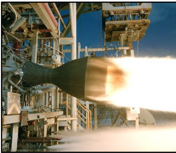
60K, Carbon Fiber Overwrapped, Chamber/Nozzle
