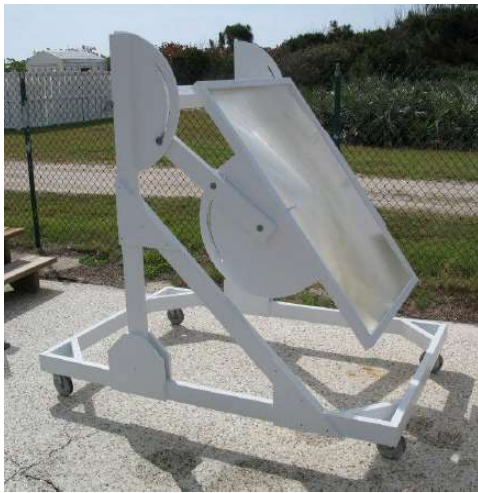
Figure 3. The 1 \text{ m}^2 solar concentrator built at NASA KSC. (credit NASA)
