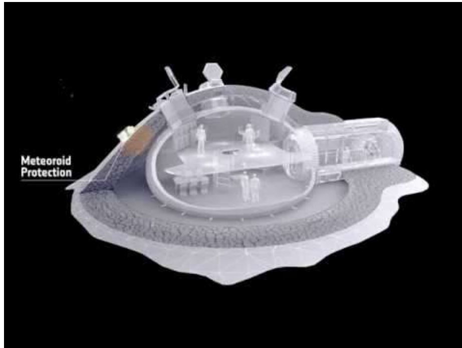
Figure 30. Cartoonist view of lunar habitat protected by regolith layer coverage from meteoroids and radiation. Image credit [86]
