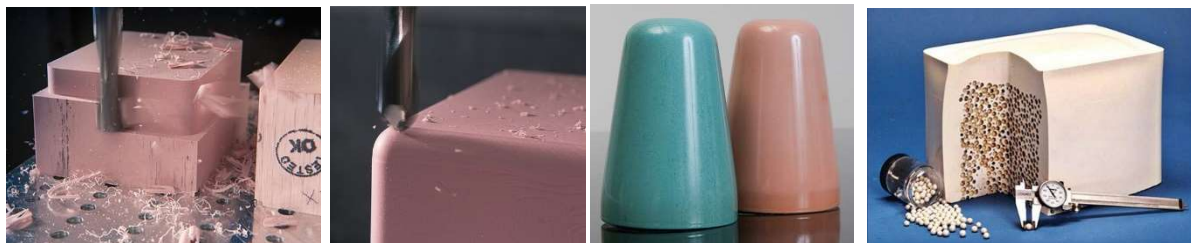
Figure 37. Syntactic foams. A fine surface finish is possible. (Courtesy CMT Plastic) [107]
