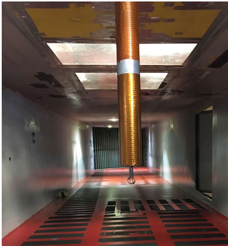
Figure 13.—Multi-Element Sensor (Science Engineering Associates, Inc.) mount without a splitter plate.
