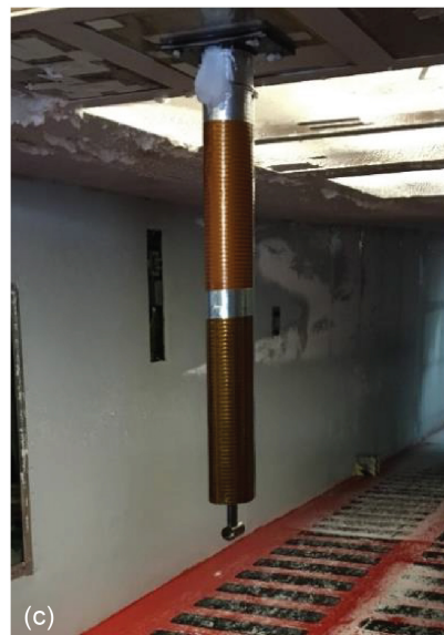
Figure 18.—Multi-wire mounting configurations tested in 2016. (a) Beveled leading edge (used in Icing Research Tunnel from 2009 to 2018). (b) Rounded leading edge. (c) No splitter plate.
