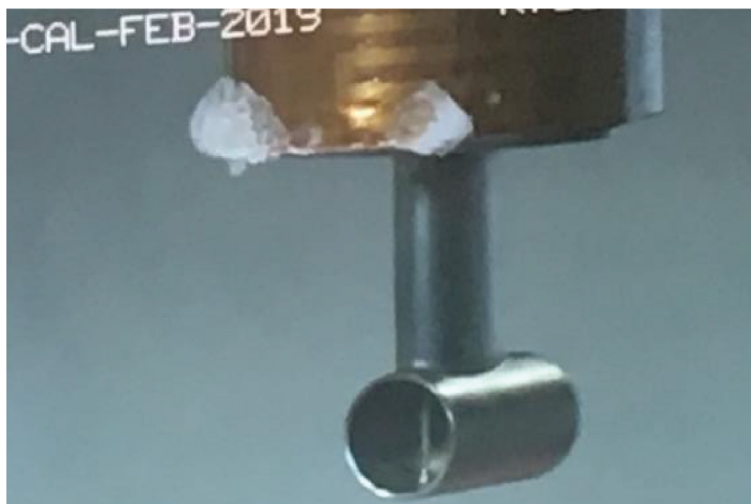
Figure 30.—Ice buildup observed on leading edge of multi-wire strut with no splitter plate.
