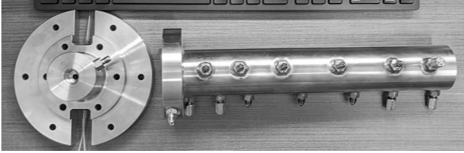
Fig. 2 - Ethane-scale test article hardware with a keyboard at the top of the photo for scale.
