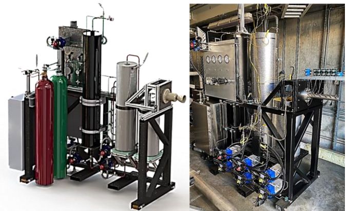
Fig. 1 - CAD model of the HPDS (left), and a photograph of the system taken during testing (right).
